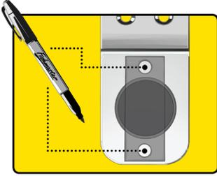
2. Drill holes through the bracket in marked areas.
