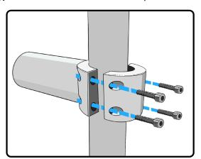
2. Place the Stabilizer Bar into the desired position on the top.
