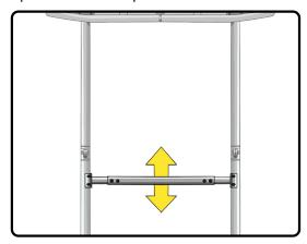
4. Make sure the bar is level before securing the other side.
